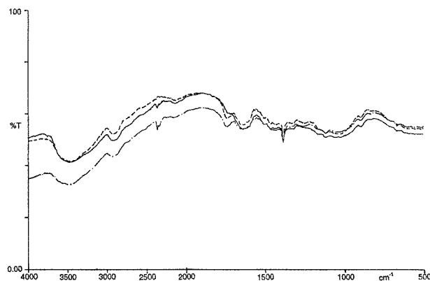
Figure 10 Infrared spectra of sisal fiber (— — —) 2% NaOH, (— · — · —) 4% NaOH, and (—) 6% NaOH.
